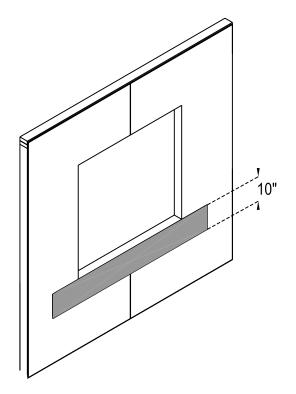
Step 1: Clean and dry substrate. Install sill flashings below openings (2 layers 60 minute grade "D" paper) 10" wide and 12" beyond side. Staple along top edge 3/8" from opening.
